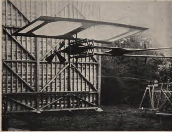
Fig. 33.—A screw and fabric covered aeroplane in position for testing.
